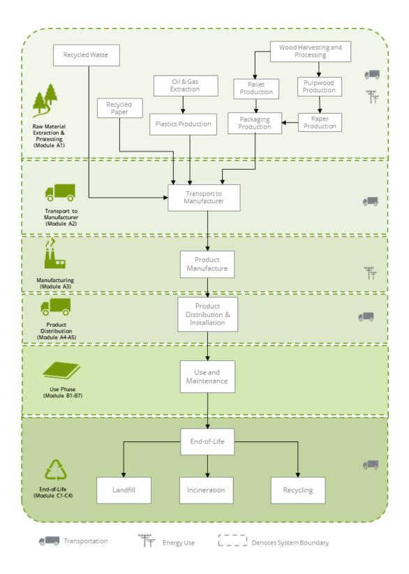
Figure 1. Flow diagram representing the major unit operations in the life cycle of the EVERBOARD™ products.
